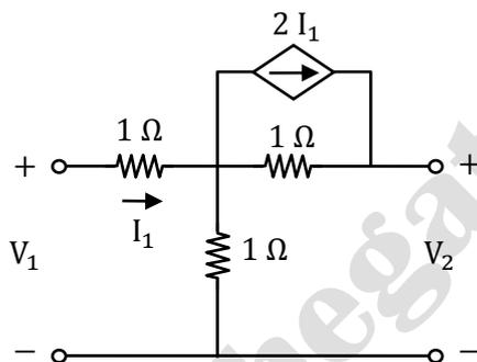
Find  $h_{11} = \frac{V_1}{I_1} \Big|_{V_2=0} ?$
